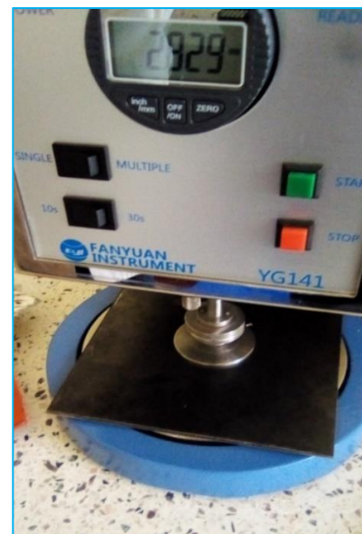
Fig. 1 Measurement of thickness using YG141 digital thickness gauge at a laboratory in the Faculty of Engineering – Busitema University.
